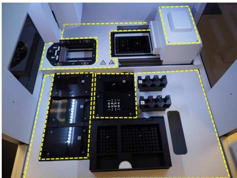
Figure 27 Deck surfaces to be wiped down
