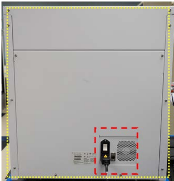
Figure 30 Exterior surfaces on the back of the instrument to be wiped down
